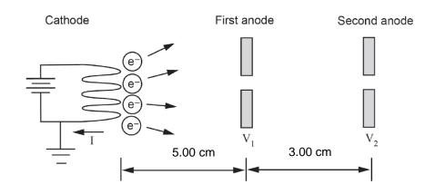
Assume the initial velocity of a thermal electron as it is emitted by the cathode is zero. The anode voltages are  $V_1$ = 1500 V and  $V_2$  = 4500 V and the distances between the cathode and anodes are as shown above.
