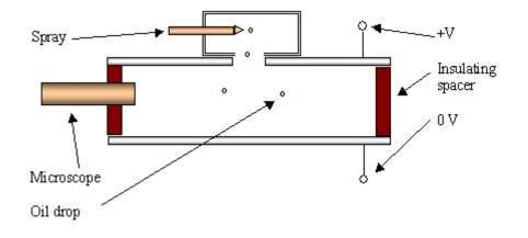
(a) If the potential difference between the plates is 7.00 kV and the plate separation is 40.0 mm, calculate electric field strength between the plates.
